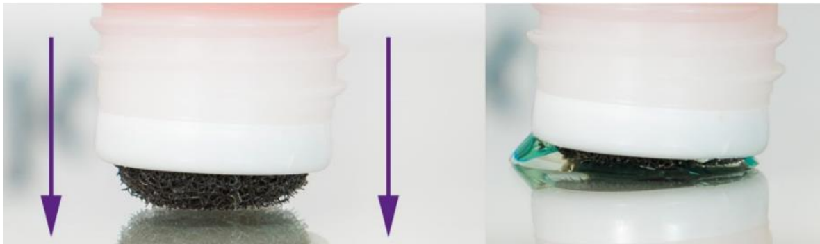
Figure 33: Depress nib on build plate to activate nozzle, Magigoo should then easily flow out!
