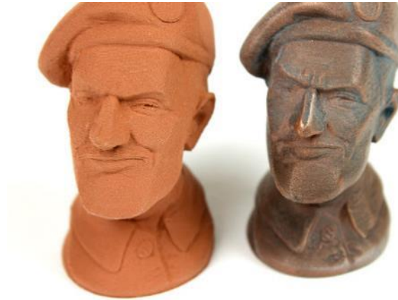
ColorFabb copperFill Metal Filament before polishing and after polishing, via: matterhackers.com
