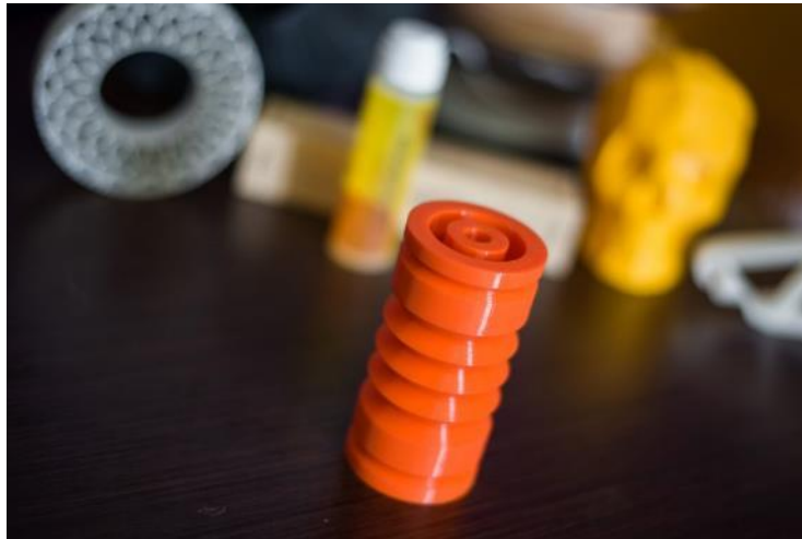
3D printed Circular Flexbellows prototype. Printed in NinjaFlex NinjaTek on a Raise3D N2 with a bondtech extruder upgrade which facilitates FDM printing of softer materials.
