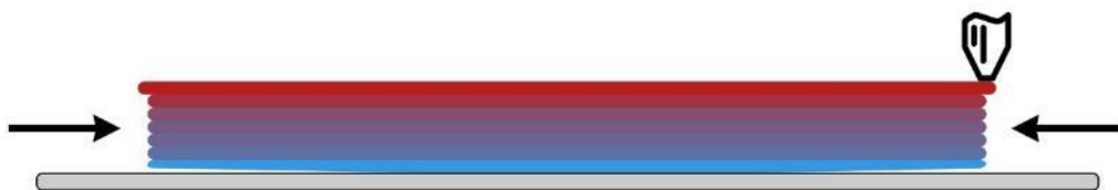
Figure 5: Print warp due to thermal gradient
