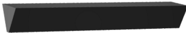
Figure 9: Wedge print, an ideal geometry for testing the first layer adhesion of your build surface, the narrow base limits the contact area with the build plate. This shape is one of the geometries used in the Magigoo testing labs to assess the adhesive performance with different material and adhesive combinations.
