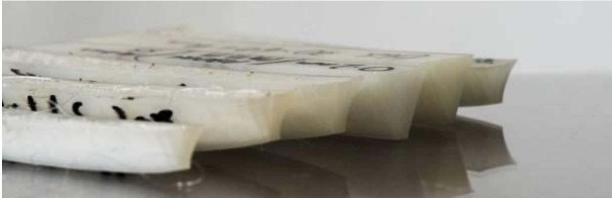
Figure 14: Wedge prints at different temperatures showing different amounts of warp and/or rates of completion
