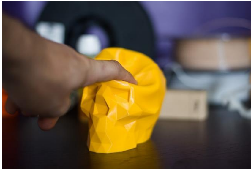
Soft materials deform easily on application of force such as this 3D print of a low poly skull. Model printed in Fillamentum Traffic Yellow TPU92A on a Raise3D N2 with a bondtech extruder upgrade which facilitates FDM printing of softer materials
